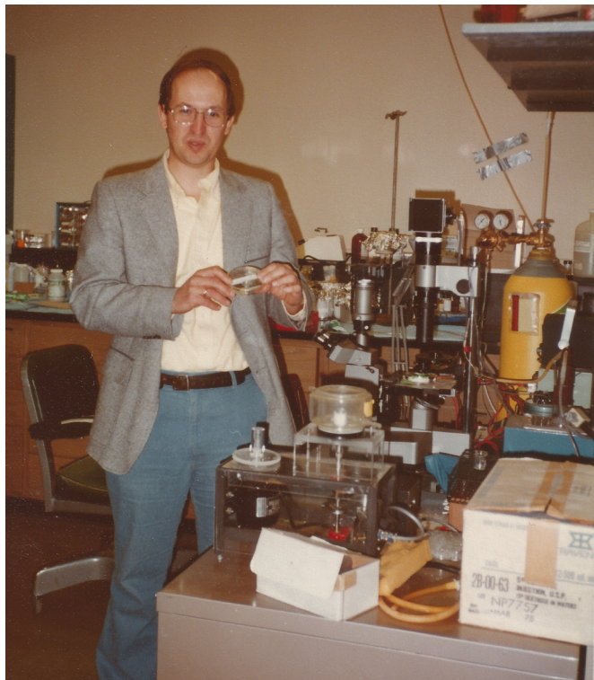
Tom Horbett was working on a spinning disc apparatus to determine critical shear stress for cell detachment.
