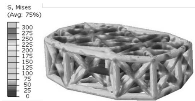
Figure 1. The Spine Truss System (STS) cage, modeled under compression, shows that the device is capable of multidimensional load bearing throughout the truss design.
