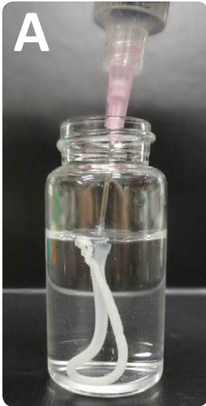
Figure 2. An injectable thermoresponsive polymer was engineered to have intrinsic antioxidant properties. The material, referred to as Nanonets™, gels at 37°C (A) and significantly inhibits lipid peroxidation, unlike commonly used materials such as polytetrafluoroethylene (ePTFE), poly(L-lactic acid) (PLLA), and poly(N isopropylacrylamide) (PNIPAAm) (B). 2
