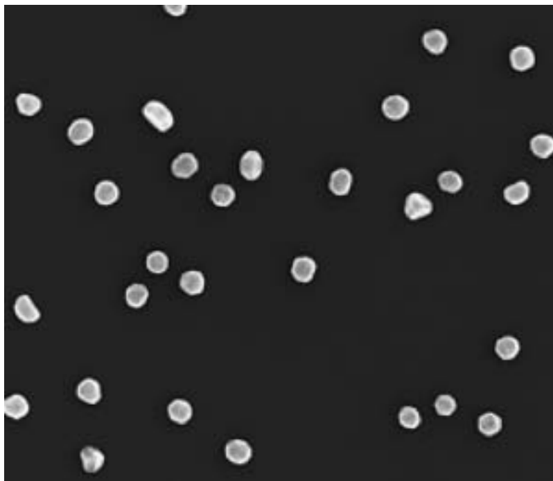
False color scanning electron micrograph (250,000 times magnification) showing the gold nanoparticles created by NIST and the National Cancer Institute’s Nanotechnology Characterization Laboratory (NCL) for use as reference standards in biomedical research laboratories.
