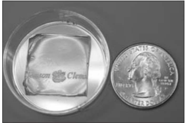
Figure 1. Precision placement of E. coli bacteria onto biopaper. Photograph of cartoon tiger paw generated by printing viable cells, according to a pre-designed pattern, onto an agar-hydrogel.
