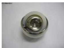
Figure 1: Acetabular shell, polyethylene liner, and femoral component of a retrieved implant
